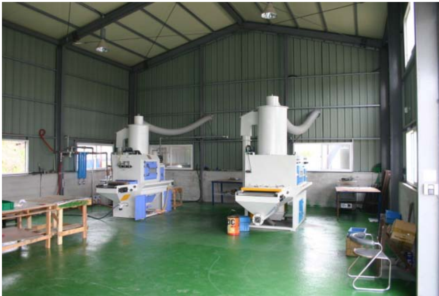
Auto Sand / Blast Machine for surface treatment of electrodes
