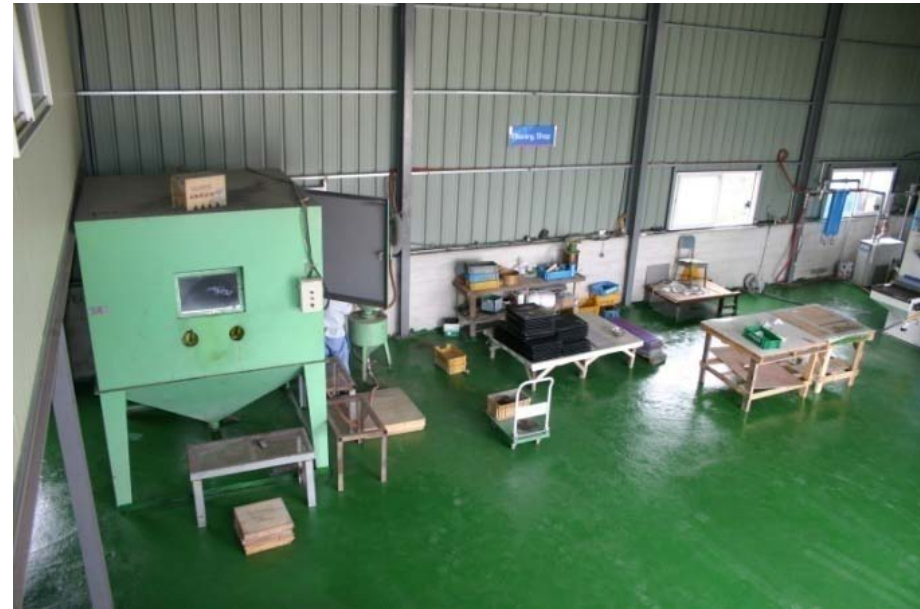
Auto Sand / Blast Machine for surface treatment of electrodes
